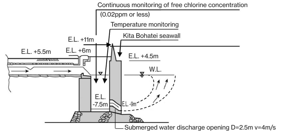
Porous dike-type submerged water discharge system
