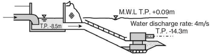
Drainpipe-type submerged water discharge system
