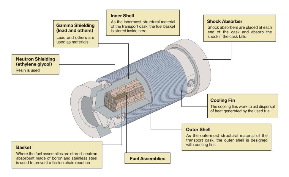
(Note) Figure shown is NFT-38B(Dry Cask) used for domestic transport.
