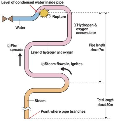
Residual heat removal system, steam condensation system pipes
