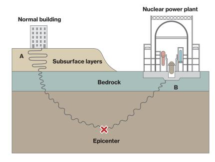
Vibration of hard ground (bedrock) is 1/3 to 1/2 that of subsurface layers.
