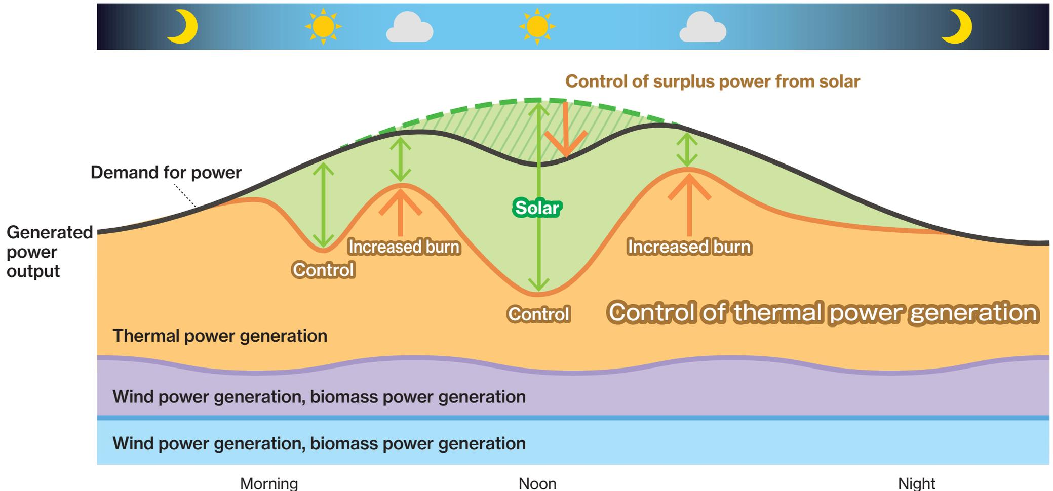
In order to achieve stable usage of power, the amount of power generated (supply) and amount of power consumed (demand) must be made always equal. For that purpose, the amount of power generated and the amount of power consumed must be balanced using methods such as thermal power generation that can compensate for the fluctuations in output from renewable energy.
