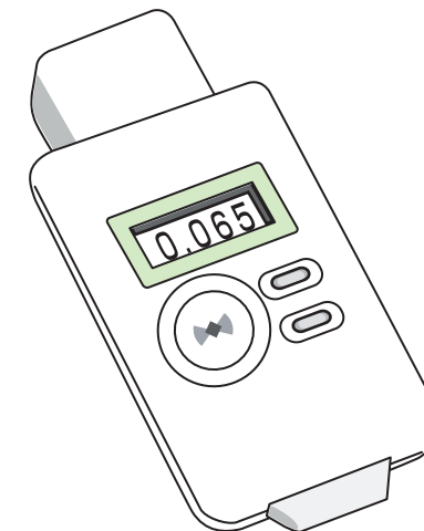
CsI Scintillation type, etc. (mainly measures low-levels)
